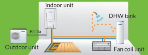
Heating and heating of DHW
