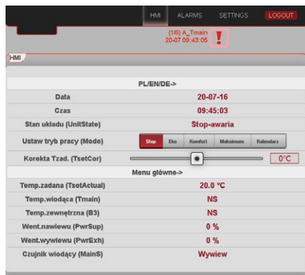
Fig. No 28 Controller HMI screen
