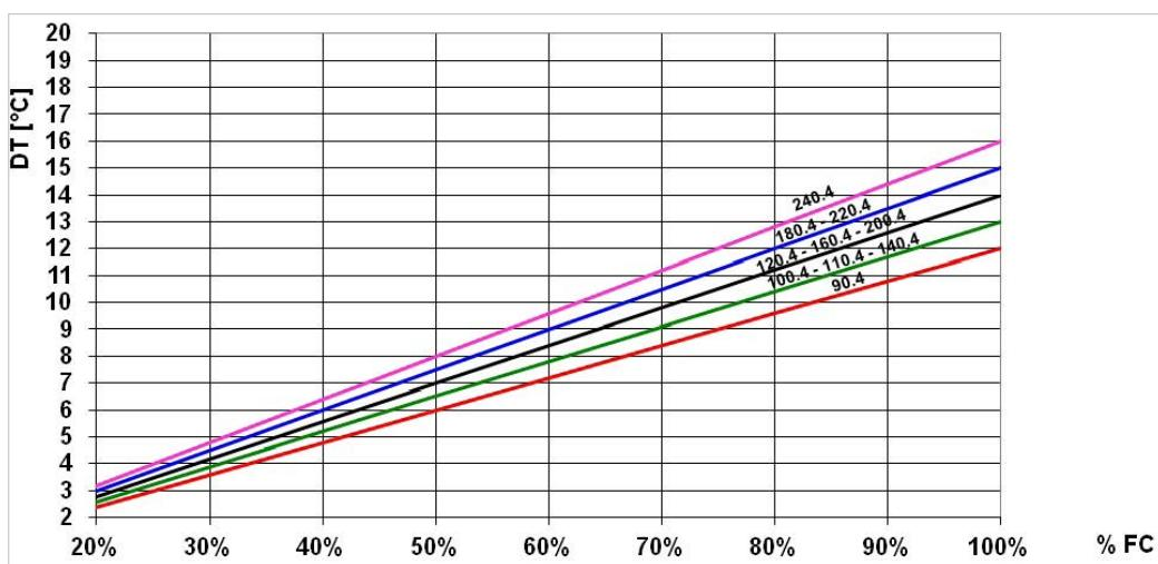
Example: Determine the performances with outdoor air = +2°C for the following unit: WSAT-XSC3 90.4 FCI EXC SC (EXCELLENCE version, No-glycol FREE-COOLING configuration), with water at 15/10 °C / 0% of glycol in the system.
