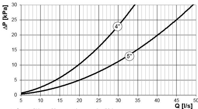
Q = water flow rate (l/s) DP = water side pressure drop (kPa)
