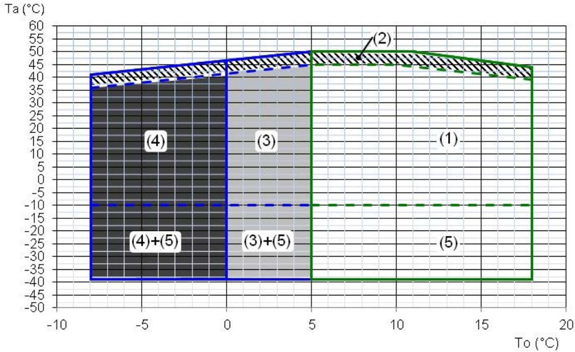
Ta (°C) = entering external exchanger air temperature (D.B.)
