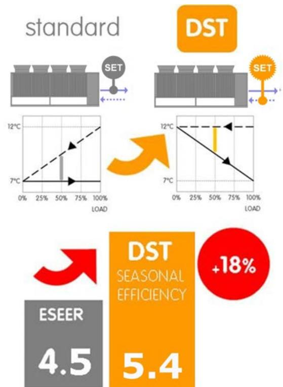
The DST control logic is as an alternative to the control logic at variable flow-rate.
