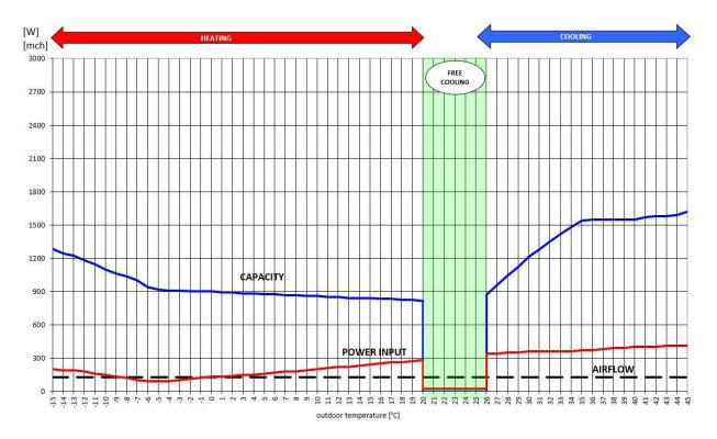
In the graph are represented the following variables: **CAPACITY** = heating / cooling capacity according to EN14511: 2018 **POWER INPUT** = Power input according to EN14511:2018 **AIRFLOW** = Room air flow rate supply [mc/h]
