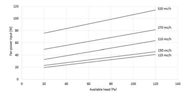
Power input raleted to the single fan in heating mode at the following conditions: Ambient temperature 7°C D.B./ 6°C W.B. Extracted air temperature 20°C D.B./ 13.7°C W.B Data with unit correct, installation and usage
