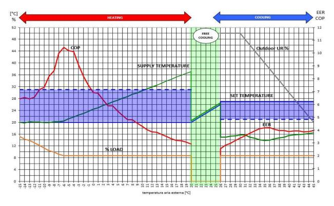
In the graphic the following variables are present: **SET TEMPERATURE** = Room set-point temperature set on remote control. **SUPPLY TEMPERATURE** = Supply air temperature from ELFOFresh EVO
