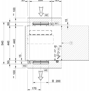
\*\* SPAZIO MINIMO PER MANUTENZIONE \*\* MINIMUN SERVICE CLEARANCE
