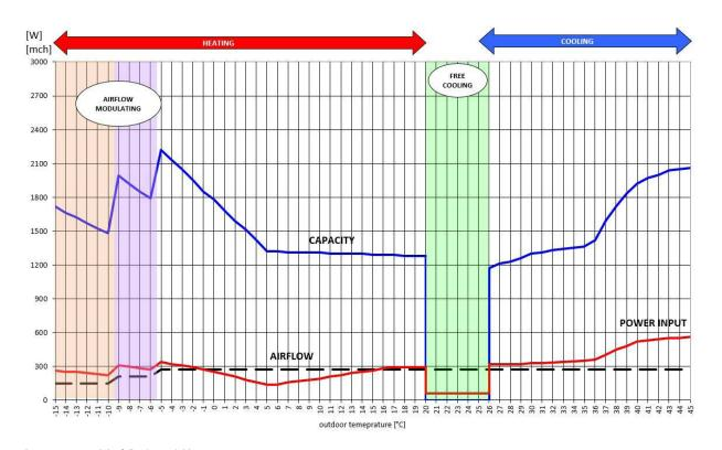
In the graph are represented the following variables: **CAPACITY** = heating / cooling capacity according to EN14511: 2018 **POWER INPUT** = Power input according to EN14511:2018
