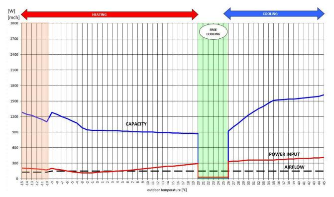
In the graph are represented the following variables: **CAPACITY** = heating / cooling capacity according to EN14511: 2018 **POWER INPUT** = Power input according to EN14511:2018
