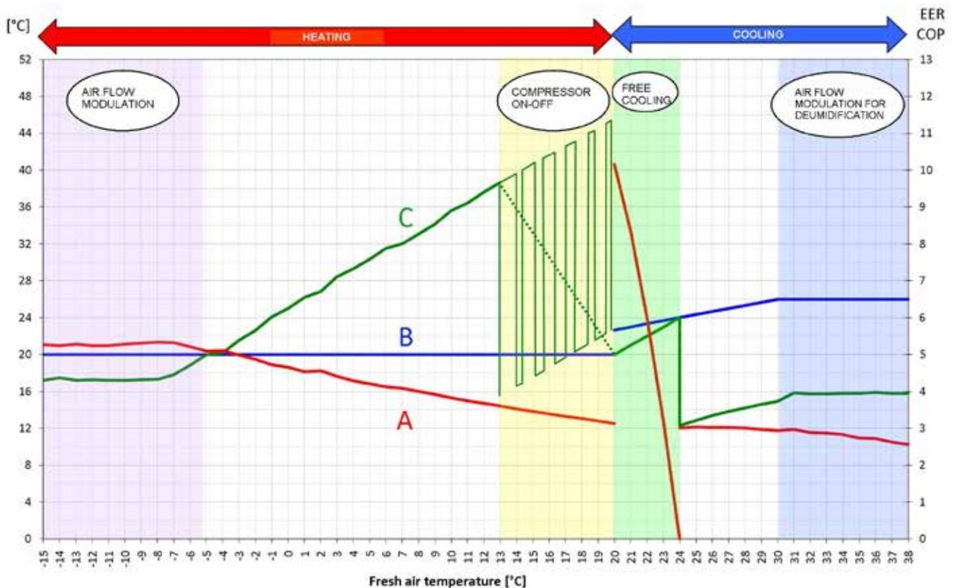
The graphic refers to size 300 and to standard set-point for a residential application and represents the trend of three variables at the fresh air temperature changing:
