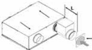
Install an air filter upstream. This should be at least a G2 class filter to protect the heating elements (provided by the customer)
