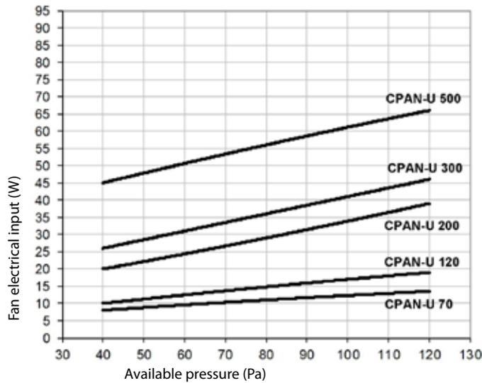
Electrical input of the single fan in conditions of standard flow in heating.
