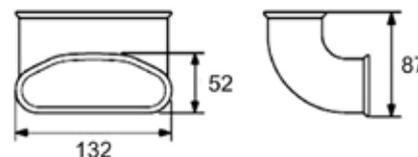
\*\*\* Joint included for flat flexible tube with double sealing ring.
