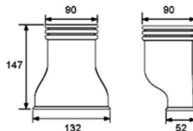
\*\*\* Joint included for flat flexible tube with double sealing ring.
