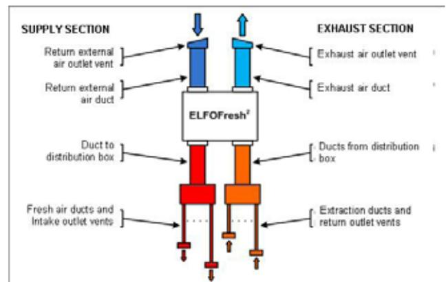
So one just needs to identify the supply and extraction duct, which features the highest pressure drops.
