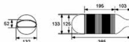
\*\*\* Joint included for flat flexible tube with double sealing ring.
