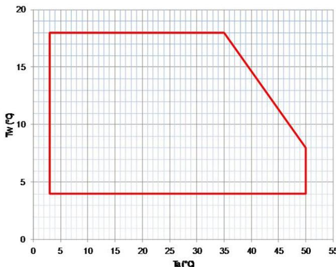
Tw [°C] = Exchanger outlet water temperature
